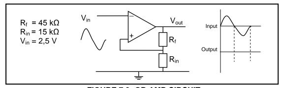
**FIGURE 7.3: OP-AMP CIRCUIT**
