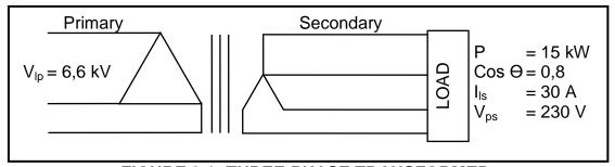
FIGURE 3.1: THREE-PHASE TRANSFORMER
