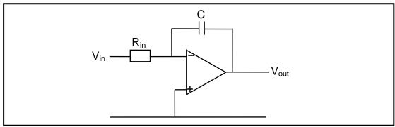
FIGURE 7.7: OP-AMP INTEGRATOR CIRCUIT
