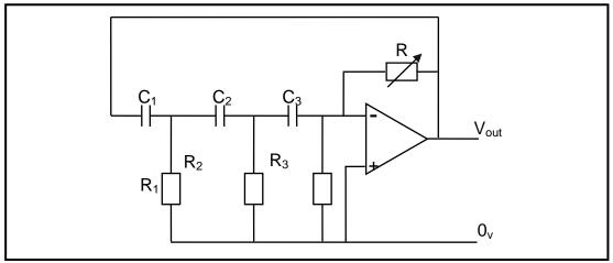
FIGURE 7.6: RC PHASE-SHIFT OSCILLATOR
