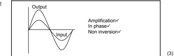
7.7.3  $AV = \frac{V_{out}}{V_{in}} = 1 + \frac{R_f}{R_{in}}$
