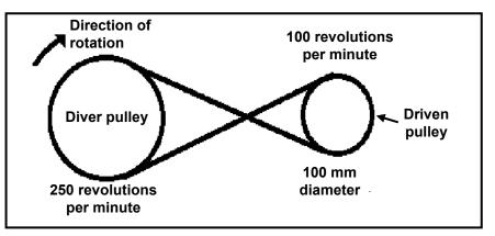
5.8.1 Calculate the diameter of the drive pulley if it turns at 25 revolutions per minute and the driven pulley turns at 100 revolutions per minute. The driven pulley has a diameter of 100 mm. Show ALL calculations.
