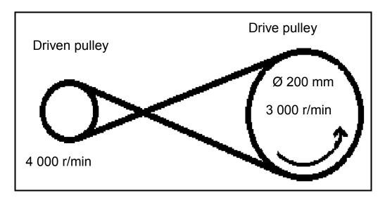
5.5.1 Calculate the diameter of the driven pulley by using the following formula:
