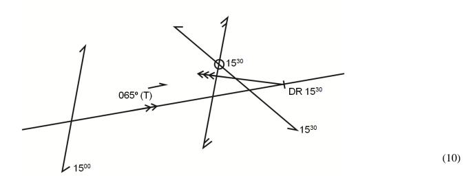
Position at 15:30 Cape Point Lt. bearing  $325^{\circ}$  (T)  $\times 2.9$  miles
