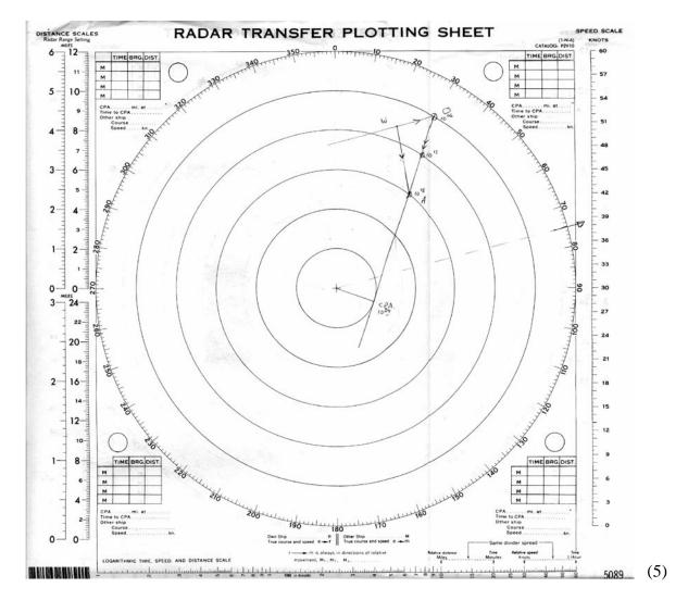
'A' 4.2 Target identification Time of initial plot 10:06 Initial range & bearing 030° (T) x 10 miles **CPA** 2,0 miles bearing 109° (T) Time of CPA 10:33 169° Target's true course (10)Target's true speed 17,5 knots.
