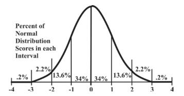
A company manufactures ball bearings. The optimum diameter of the spherical bearing is 42 mm. Records show that the diameter follows a normal distribution with a mean of 42 mm and a standard deviation of 0,06 mm. A diameter of 41,94 mm and 42,06 mm is acceptable.
