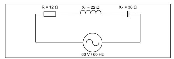
FIGURE 2.3: RLC SERIES CIRCUIT
