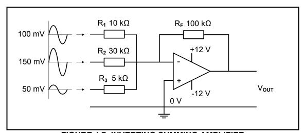
FIGURE 4.7: INVERTING SUMMING AMPLIFIER
