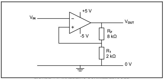
FIGURE 4.5: INVERTING SCHMITT TRIGGER
