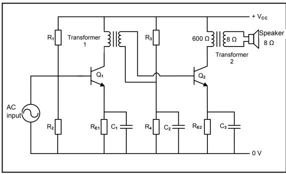
FIGURE 5.5: TRANSFORMER-COUPLED AMPLIFIER
