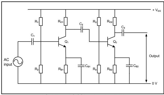
FIGURE 5.3: RC-COUPLED AMPLIFIER
