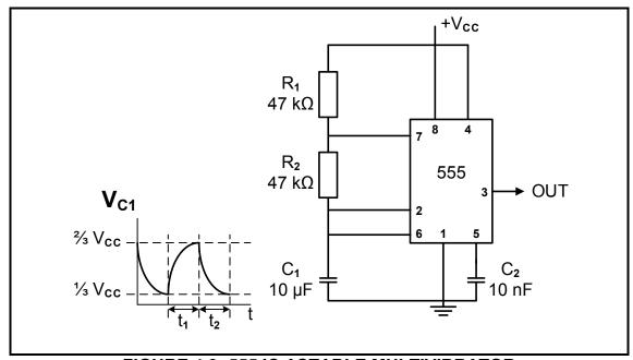
FIGURE 4.3: 555 IC ASTABLE MULTIVIBRATOR
