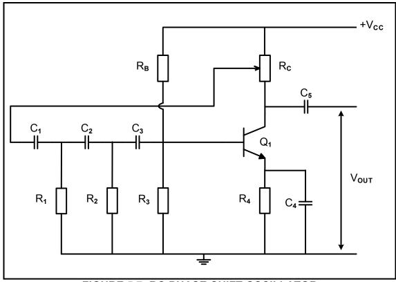
FIGURE 5.7: RC-PHASE-SHIFT OSCILLATOR
