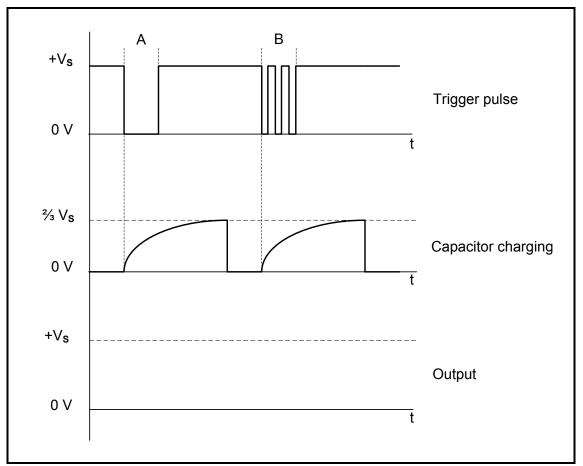
FIGURE 4.4: MONOSTABLE MULTIVIBRATOR TRIGGER PULSES
