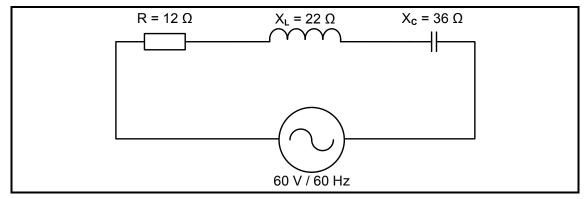
FIGURE 2.3: RLC SERIES CIRCUIT
