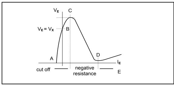
FIGURE 3.4: UJT CHARACTERISTIC CURVE
