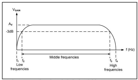
FIGURE 5.4: FREQUENCY RESPONSE OF RC-COUPLED AMPLIFIER
