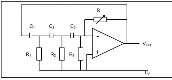
FIGURE 7.5: RC PHASE-SHIFT OSCILLATOR
