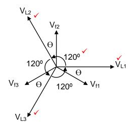
One mark for showing  $V_{ph}$  is smaller than  $V_{L}\checkmark$   $V_{ph}$  lags  $V_{L}\checkmark$  by  $\Theta$ =30 degrees
