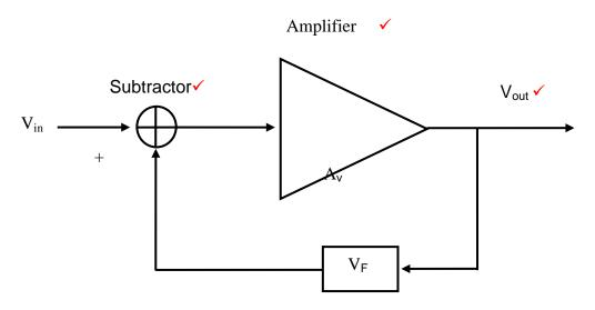
Feedback Network√ out of phase with the input.
