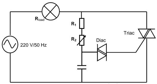
FIGURE 6.1: LAMP DIMMING CIRCUIT
