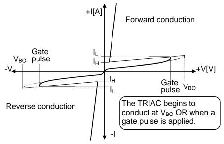
FIGURE 6.2: CHARACTERISTIC CURVE OF A TRIAC
