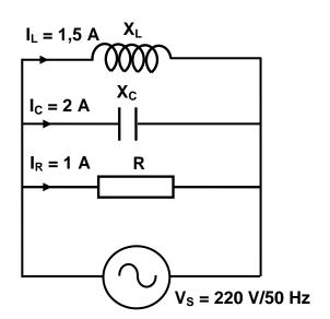
FIGURE 5.1: PARALLEL RLC CIRCUIT [30]
