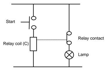
FIGURE 9.1: RELAY CIRCUIT
