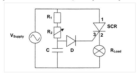
FIGURE 6.2: LAMP-DIMMING CIRCUIT
