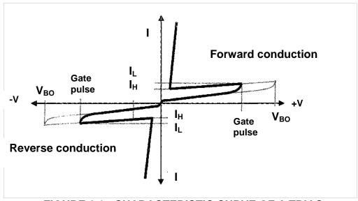
FIGURE 6.1: CHARACTERISTIC CURVE OF A TRIAC
