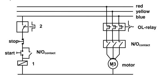
FIGURE 10.1: DIRECT-ON-LINE-STARTER
