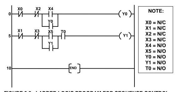
FIGURE 9.2: LADDER LOGIC PROGRAM FOR SEQUENCE CONTROL
