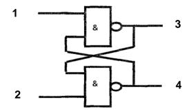
FIGURE 9.1: CIRCUIT OF A LATCH
