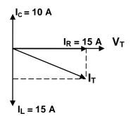
FIGURE 5.1: PHASOR DIAGRAM OF AN RLC PARALLEL CIRCUIT
