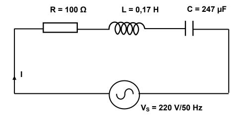
FIGURE 5.1: RLC SERIES CIRCUIT
