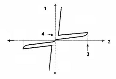
FIGURE 6.1: CHARACTERISTIC CURVE OF A DIAC
