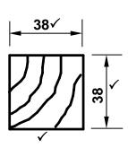
Batten 38 mm x 38 mm/ 50 mm x 38 mm tilting batten For concrete roof tiles
