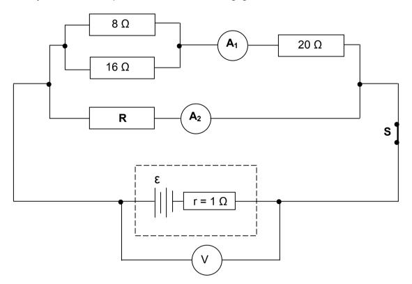
With switch **S** closed, the current passing through the 8  $\Omega$  resistor is 0,5 A.
