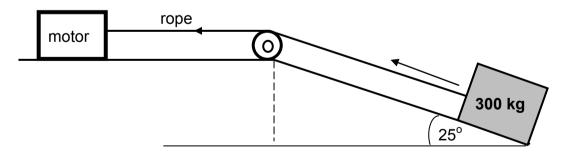
5.2.1 Calculate the magnitude of the frictional force acting between the crate and the surface of the inclined plane. (3)
