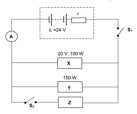
With switch  $S_1$  closed and  $S_2$  open, the devices function as rated.
