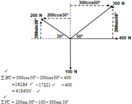
$\sum VC = 200 \sin 30^{\circ} - 100 + 300 \sin 50^{\circ}$ =  $100 \checkmark -100 + 229.81 \checkmark$ =  $229.81N \checkmark$
